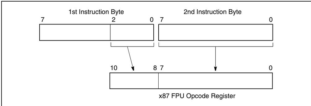
**Figure 8-8. Contents of x87 FPU Opcode Registers**
