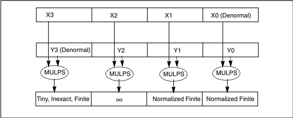
Figure 11-9. Example Masked Response for Packed Operations
