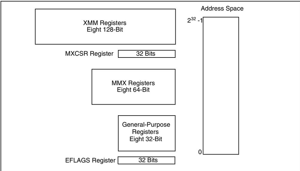
Figure 11-1. Streaming SIMD Extensions 2 Execution Environment
